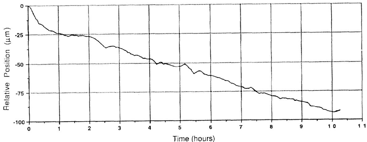
Figure 4. Example of vertical position drift of a stored 2GeV beam. The starting current is 190mA and the final current 125mA.
