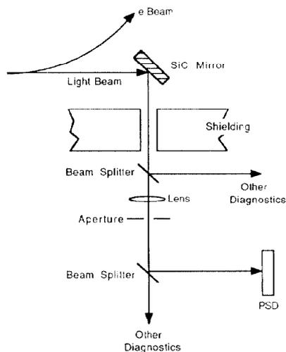
Figure 1. Schematic layout of the synchrotron light area.
