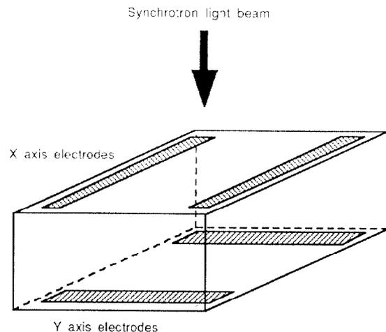
Figure 2. Sketch of the photodetector head.
