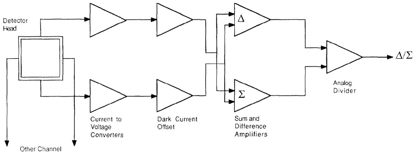
Figure 3. Schematic of the signal processing electronics.
