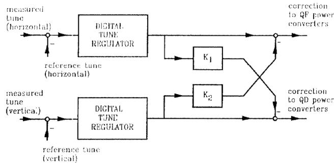
Fig. 5 Closed loop tune regulation
