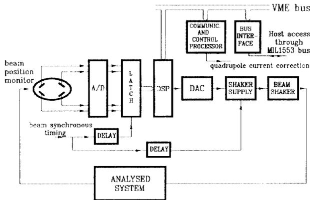
Fig. 1 Hardware components: Beam position measurement, signal processor (DSP) and beam shaker.
