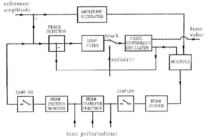
Fig. 3 Signal flow diagram for PLL mode.
