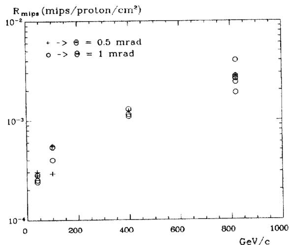
Figure 1: Rate of minimum ionizing shower particles crossing an area of  $1 \text{ cm}^2$  at the downstream end of the quadrupole.  $\theta$  is the angle of the incident proton.
