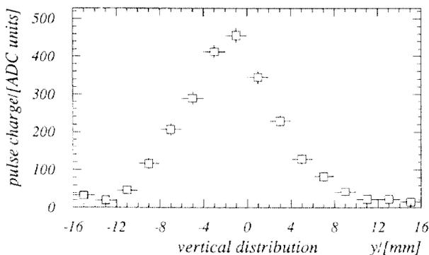
Figure 6: Vertical profile of the backscattered photons
