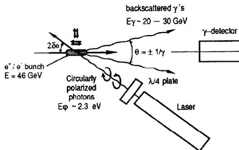
Figure 1: Principle of the laser polarimeter
