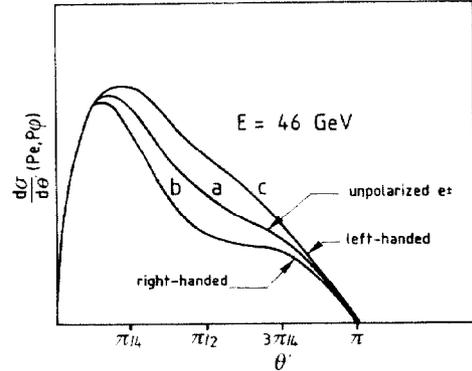
Figure 2: Spin-dependent Compton cross section vs. scattering angle  $\theta'$  in the  $e^\pm$  rest frame for right- and left-handed circularly polarized photons on 46 GeV vertically polarized leptons.
