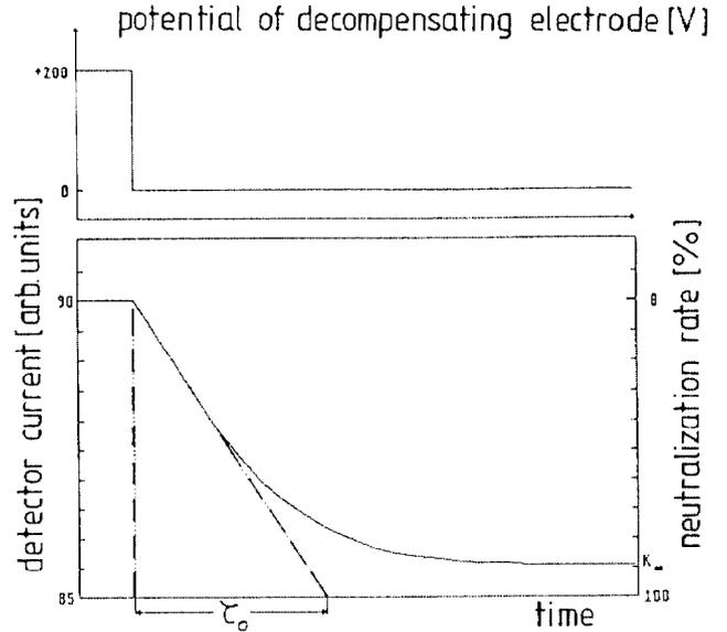
Fig 6 : Time evolution of the space charge compensation rate (schematic)
