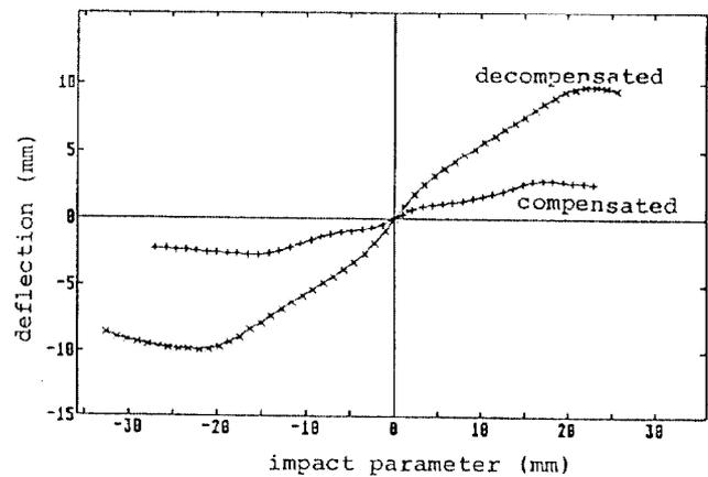
Fig 3 : Deflection characteristics of a neutralized and a decompensated  $Ar^+$  beam (0.8 mA, 10keV)
