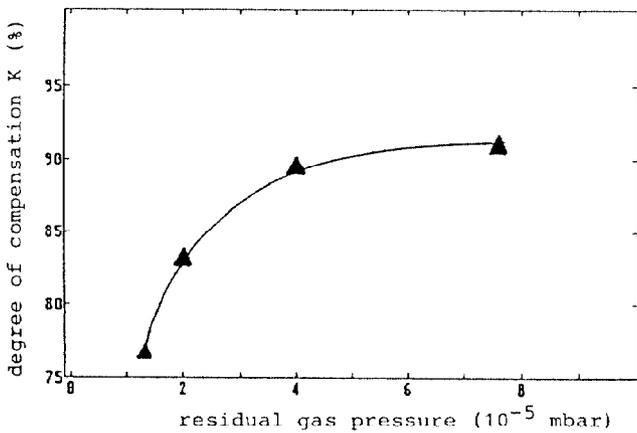
Fig 5 : Measured degrees of compensation versus residual gas pressure
