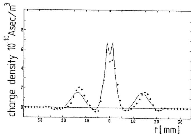
Fig 4 : Radial net charge density distribution of a compensated  $Ar^+$  ion beam
