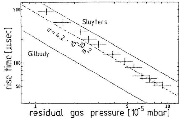
Fig 7 : Measured minimum rise times versus residual gas pressure for a 10 kev, 0.8 mA,  $Ar^+$  beam. The dashed line corresponds to a  $\sigma_i$  measured at high pressure; the solid lines refer to values of  $\sigma_i$  from literature [6,7]. The decreasing cross section for low pressures is due to the increasing hydrogen component in the residual gas mixture.
