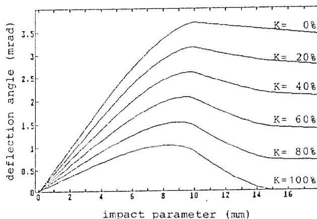
Fig 2 : Calculated deflection characteristics for different degrees of compensation.
