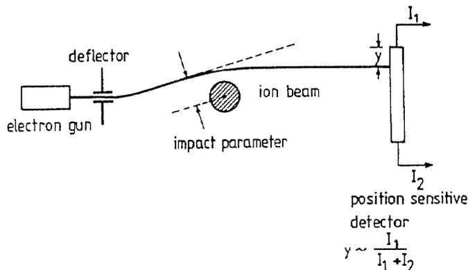
Fig 1 : Schematic layout of the experimental setup
