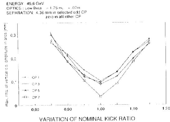
fig. 2: Dependence of vertical c. o. rms outside separator bump from the kick ratio for odd CPs
