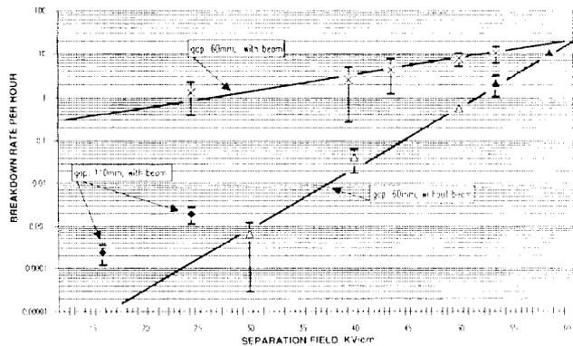
fig. 4: Breakdown rate per separator unit as a function of mean electric field strength
