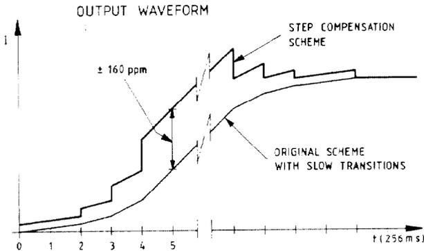
Fig. 4 - Compensation of the effects of the dipole vacuum chamber eddy currents by adding current offsets in the PC's of the quadrupole and sextupole circuits .
