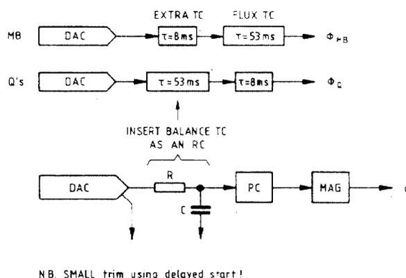
Fig. 3 - Balancing time-constants
