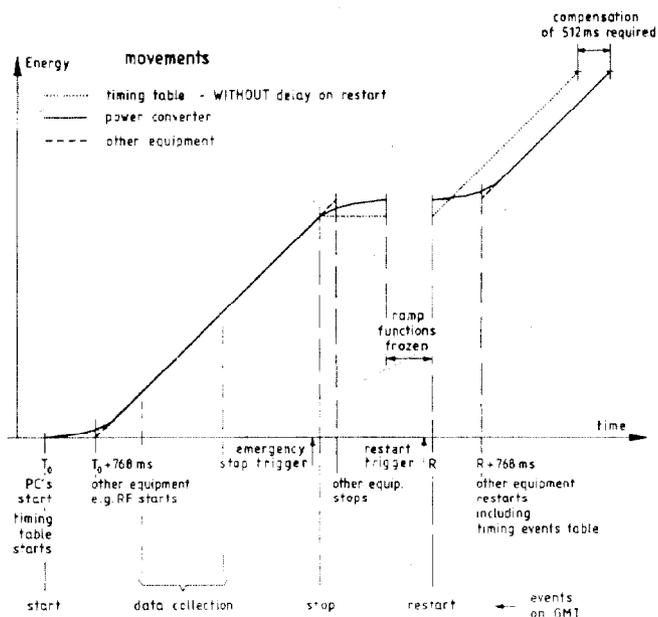
Fig. 1 - Timing events and equipment synchronization
