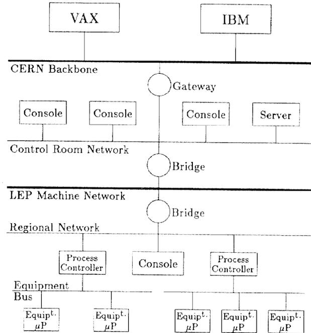
Figure 1: LEP Control System Networks
