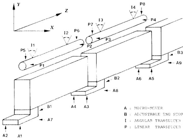
Fig. 3 Support, movement and measurement system
