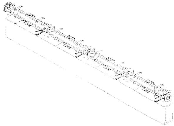
Fig. 1 Conceptual design of the CLIC accelerating structure
