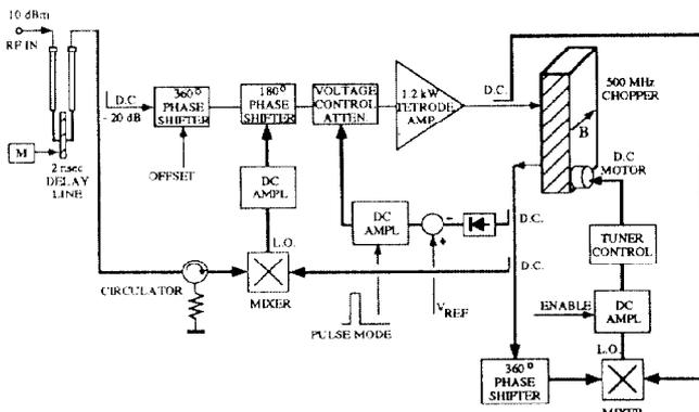
FIG. 4 - Schematic Block Diagram of the 500 MHz Chopper System.
