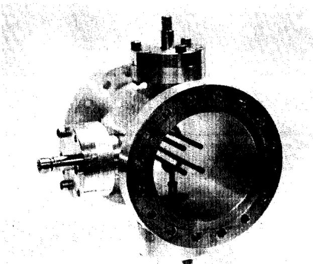
Fig. 2 - The 50 MHz Sub-Harmonic chopper.
