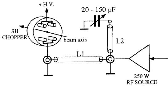
FIG. 3 - Schematic Layout of the 50 MHz Sub-Harmonic Chopper.
