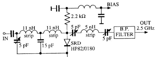
FIG. 7 - Circuit of the Step Recovery Diode Frequency Multiplier.
