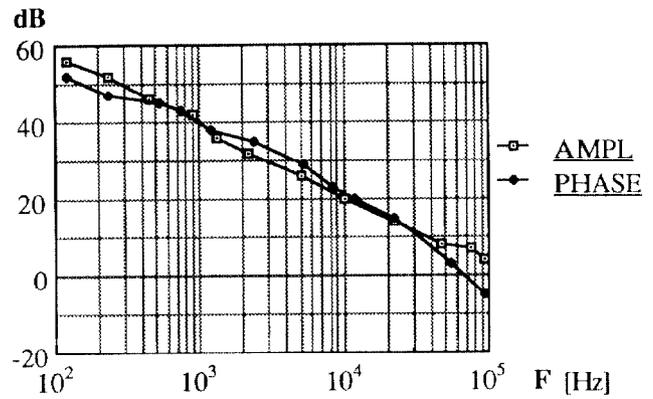
Fig.5 - Bode Diagrams of the Feedback Transfer Functions for the 500 MHz chopper.
