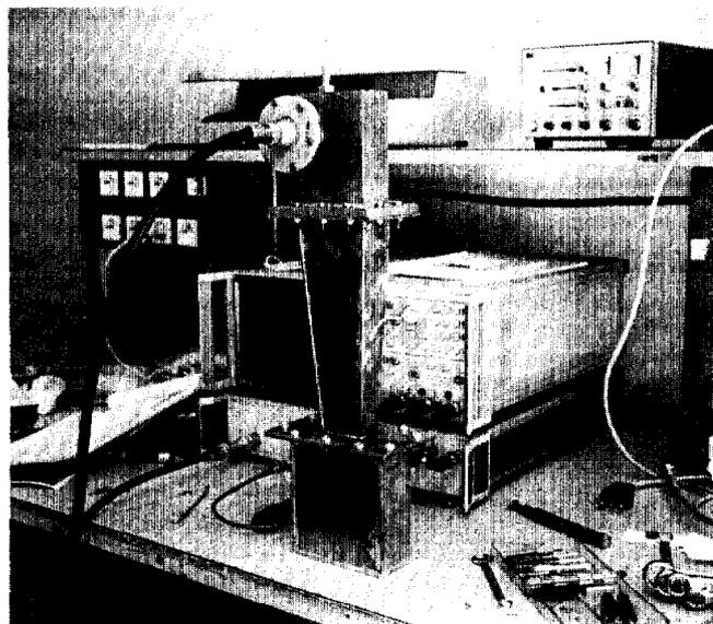
Fig.8 - RF test of a prototype of the deflecting cavity for the bunch length measurement.
