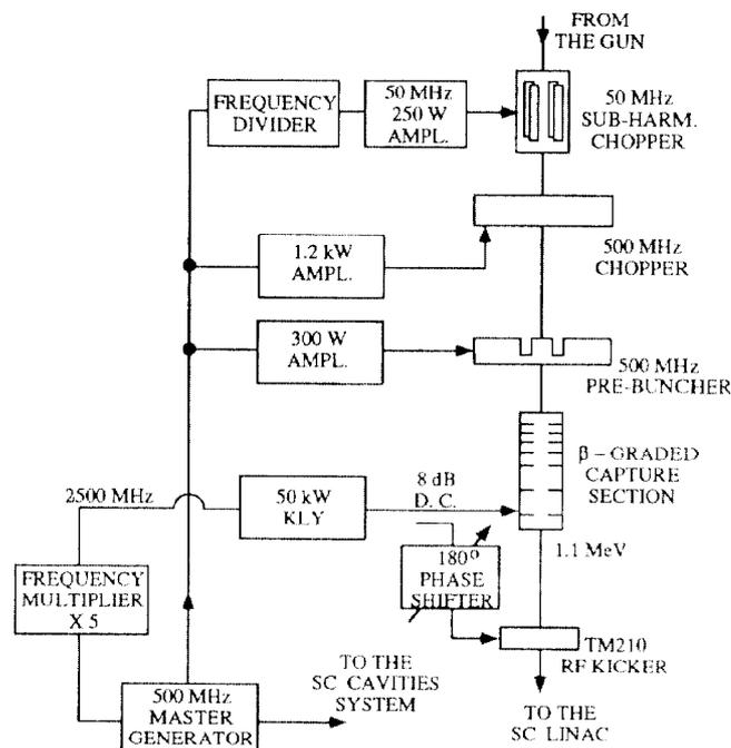
FIG. 1 - Layout of the Injector RF System.
