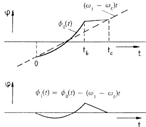
Fig. 5: Relationship between phase and frequency modulation
