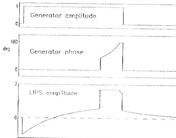
Fig. 3: Waveforms of the continuous-phase SLED
