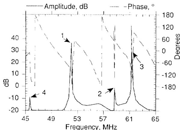
Fig. 5. HERA Fast Loop Bode Plot.
