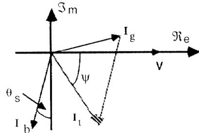
Fig. 2. Phasor Diagram in 52 MHz Frame of Reference.
