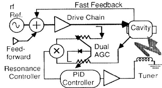
Fig. 1. Fast Loop, Feedforward and Resonance Controller.
