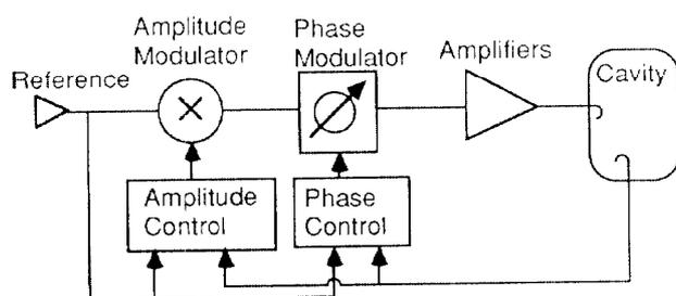
Fig. 3. Separate Amplitude and Phase Loops.
