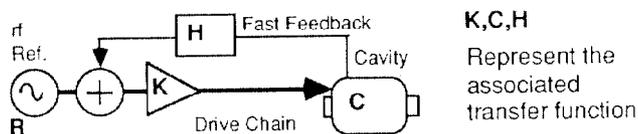
Fig. 4. Basic Components of Direct Feedback.
