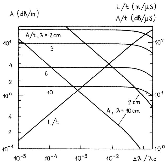
Fig. 1. Plots of power dissipation  $A$ , normalized dissipation  $A/t$  and normalized length  $L/t$  as a function of  $\Delta\lambda/\lambda_c$  for different values of  $\lambda$  for rectangular waveguide.
