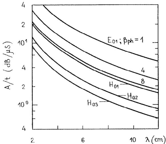
Fig. 4. Plots of normalized power dissipation  $A/t$  as a function of wavelength  $\lambda$  for different modes in CIW.
