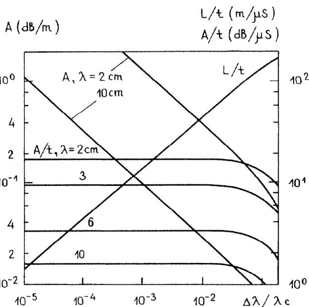
Fig. 2. Plots of values  $A$ ,  $A/t$  and  $L/t$  as a function of  $\Delta\lambda/\lambda_c$  parameter for circular smooth waveguide.
