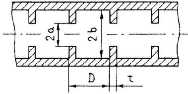
Fig. 3. Circular iris-loaded waveguide structure.
