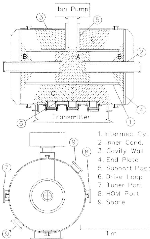
Fig. 1 Outline of HERA 52 MHz cavity. Areas A, B, and C indicate titanium deposition.
