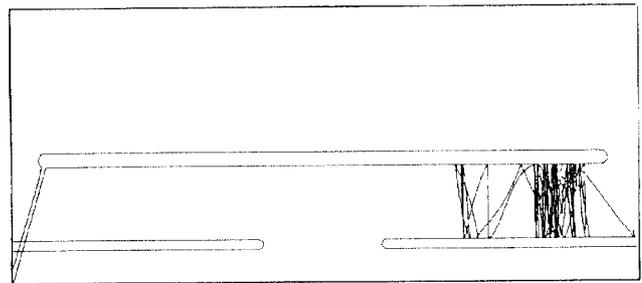
Fig. 2 Half-section model of HERA cavity showing resonant trajectory for  $V_{\text{GAP}} = 7.4 \text{ kV}$ .
