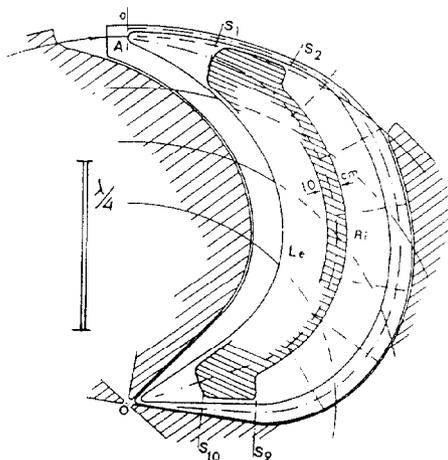
Fig. 2. The Eulima cavity. Horizontal section at  $3/4$  h.
