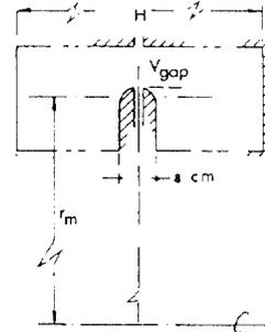
Fig. 3. Cross-section of the conducting waveguide.
