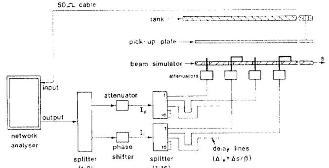
Fig. 3 : Measurement set-up (schematic).
