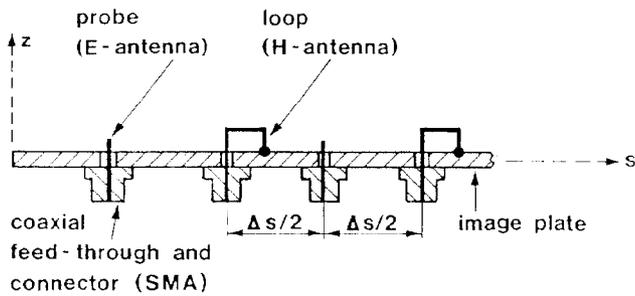
Fig. 1 : Cross-section of the beam-simulator.
