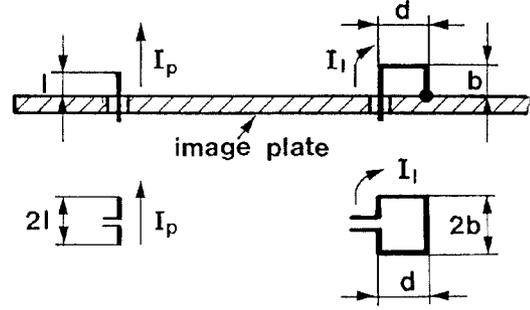
Fig. 5 : Probe and loop on image plate (a) and equivalent sources in free space (b).
