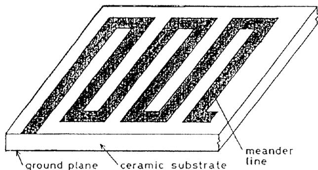
Fig. 7: Sketch of the meander pick-up (adapted from [4]). Only the lower electrode is shown.
