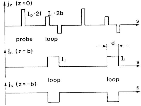
Fig. 6.: Vertical and longitudinal current sources produced by the beam simulator.
