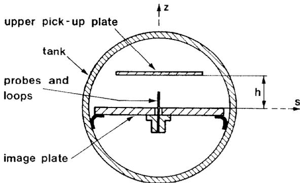
Fig. 2 : Beam-simulator installed in pick-up tank.
