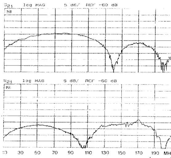
Fig. 8 Sensitivity of meander coupler (upper curve) and loop coupler v.s. frequency. Vertical scale: 5 db/division
