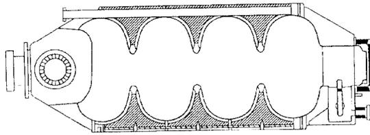
Fig. 1: Layout of the 4-cell 500 MHz cavities for HERA
