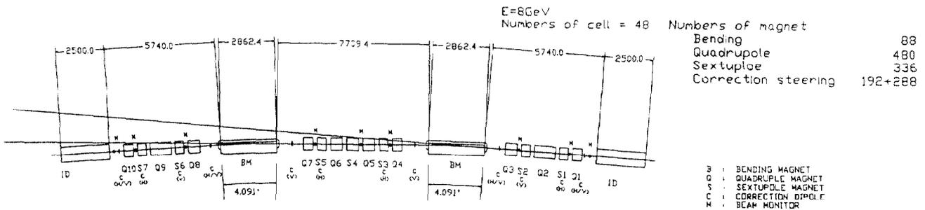
Fig.1. Layout of lattice main magnets for 1 cell of the 8 GeV storage ring.
