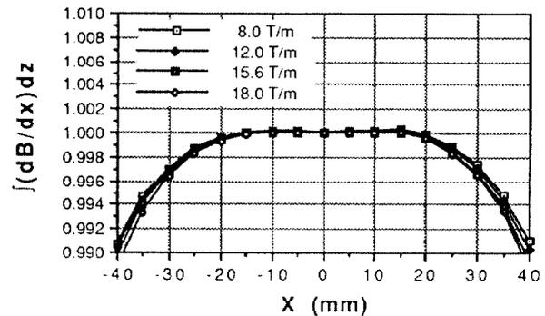
Fig.7. Transverse distributions of integrated field gradients of a prototype quadrupole magnet.
