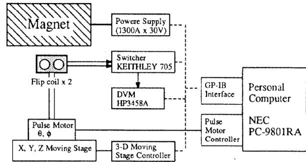
Fig.6. Block diagram of field measurements system.
