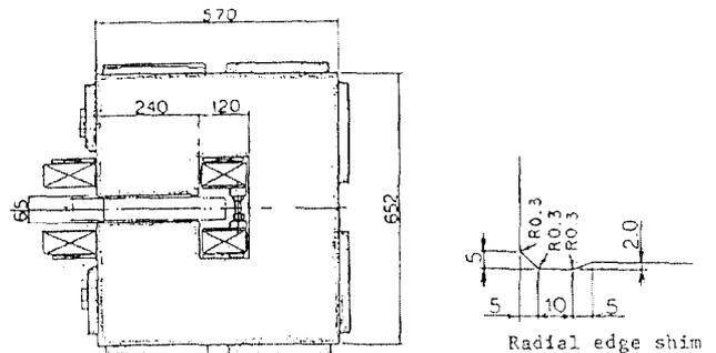
Fig.2. Cross-sectional view of a dipole magnet.
