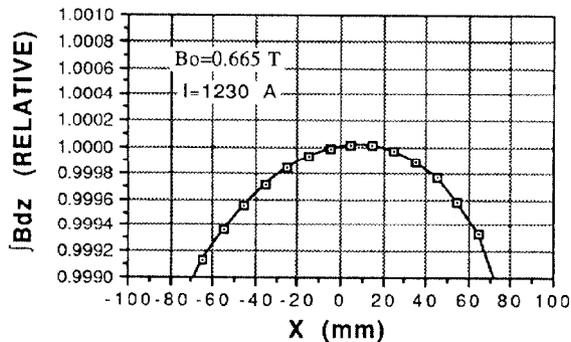
Fig.5. Transverse distribution of field integration of a prototype dipole magnet.
