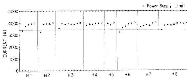
Fig 3. Training history of eight quadrupoles. The black circles and the black triangle indicate inner coil quenches and outer coil quenches, respectively. The white circles indicate no quenches.
