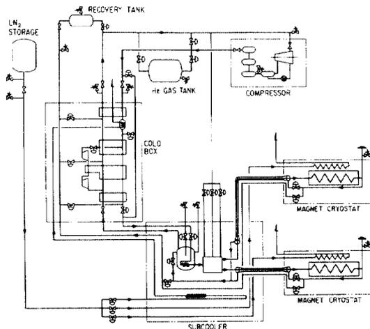
Fig 6. Flow diagram of the cryogenic system.
