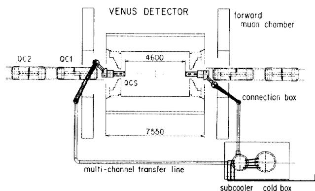
Fig. 1. Layout of the superconducting quadrupole system near an experimental detector of TRISTAN. QC1 and 2 are conventional quadrupoles. They have been used to obtain higher luminosity until the installation of the superconducting quadrupole(QCS) is completed. After installation, QC1 and QCS will be used to squeeze the beam at the collision point and even higher luminosity will be obtained.
