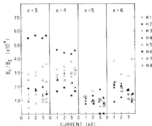
Fig 4. Harmonic content of the integrated magnetic field.
