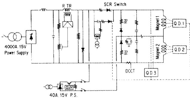
Fig 5. Electric circuit of the superconducting magnet system.
