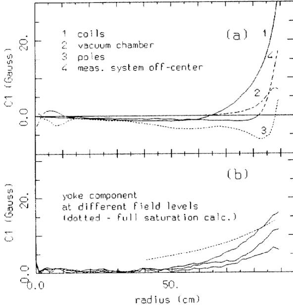
Fig.4: a) 1<sup>st</sup>harmonic components for map at 1750/1750 (4.8 Tesla). The lower graph shows the increase of the yoke contribution with the field (3.8, 4.3 and 4.8 Tesla), compared with the calculated one at maximum field.
