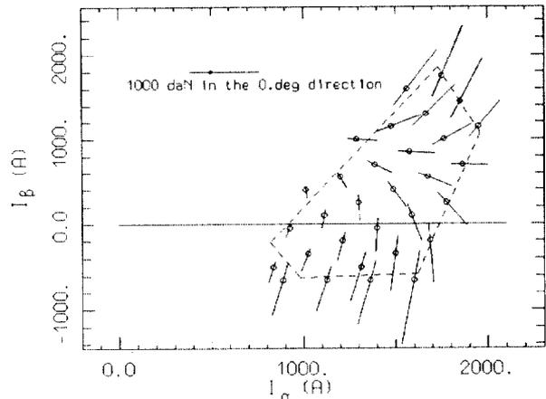
Fig.5: Forces acting on coils at the grid points. The bar orientation gives the force direction when  $I_\alpha$  is the x-axis and  $I_\beta$  is the y-axis.
