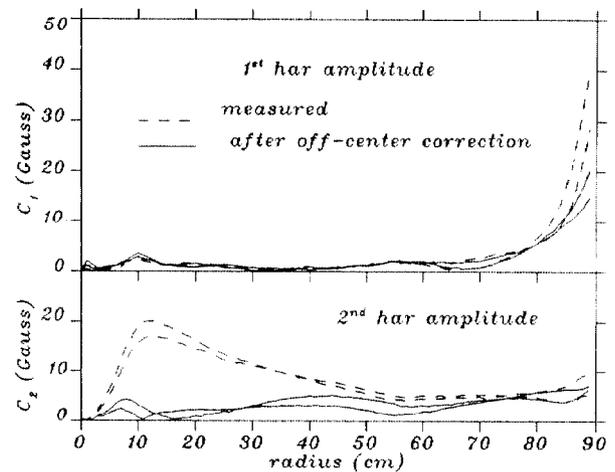
Fig.2: 1<sup>st</sup> and 2<sup>nd</sup> harmonic amplitudes vs radius.
