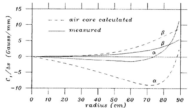
Fig.3: measured (solid lines) 1<sup>st</sup> harmonic given by coil displacement compared with the air core calculation, for  $\Delta s = 1$  mm and  $I_\alpha = I_\beta = 1000$  A.
