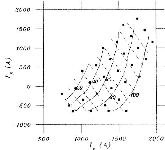
Fig.1: operating diagram with the mapping grid. Contour lines of the magnetic flux (dashed) and of the difference in  $3^{rd}$  harmonic amplitude (Gauss) at radius 72 cm.
