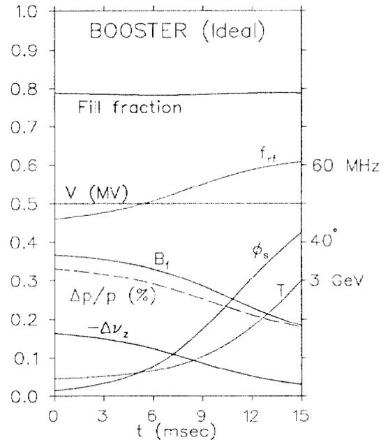
Fig. 4. Bunch parameters during the Booster cycle for the "ideal" magnet waveform giving constant bucket area for constant rf voltage.
