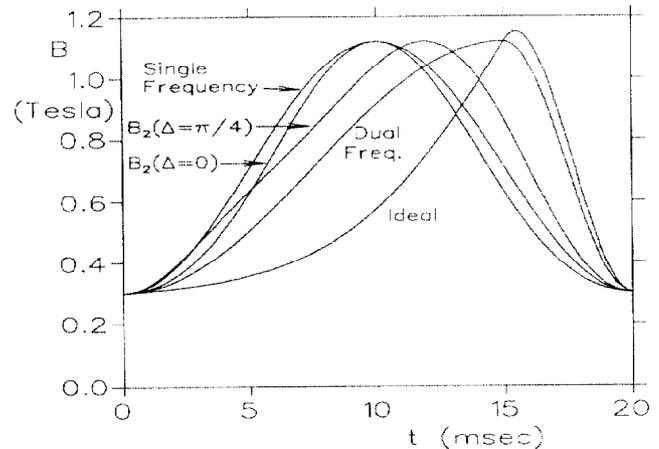
Fig. 3. Various magnetic field waveforms considered for the Booster.
