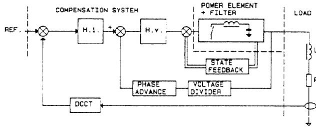
Fig. 2 Closed-loop system for a converter with a magnet
