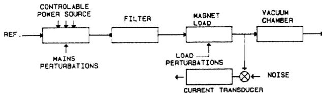
Fig. 1 Block diagram of a power converter
