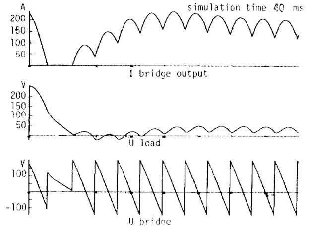
Fig. 3 Lost of conduction of a thyristor bridge
