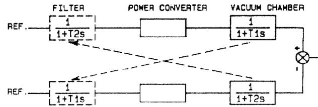
Fig. 5 Block diagram of dipole and quadrupole systems
