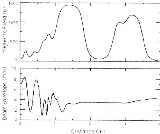
Fig.1 Magnetic field variation and beam envelope from the gun to the end of the first accelerating column
