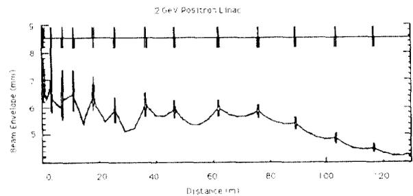
Fig.4 Typical beam envelope for 2 GeV positron
