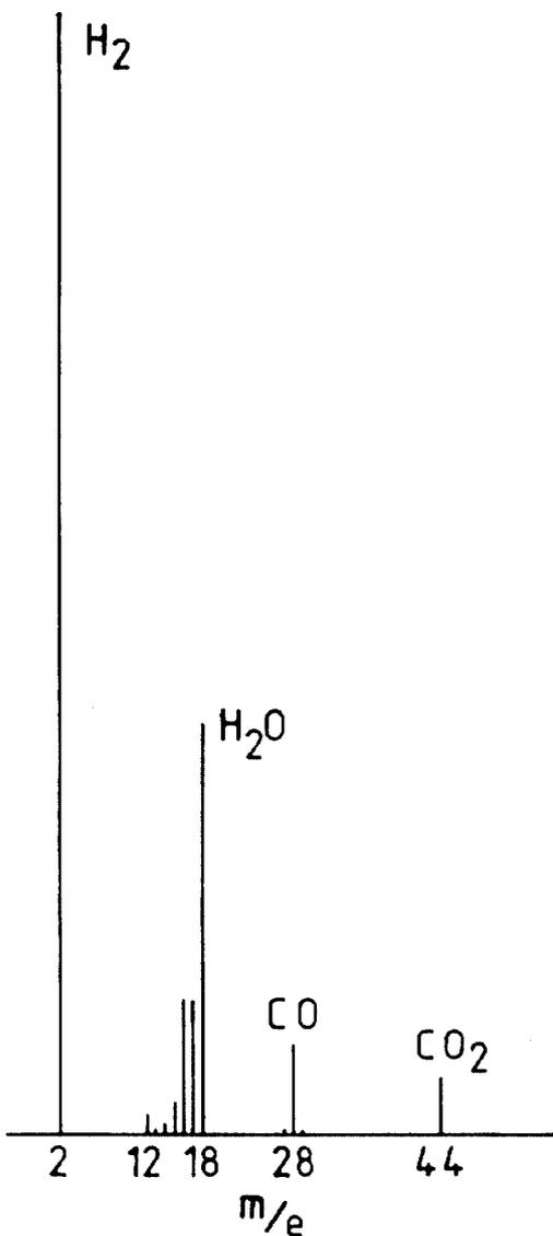
Fig. 3 : The residual gas spectrum in an unpowered cavity assembly.
