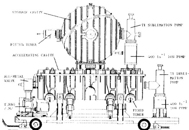
Fig. 1: An RF cavity assembly on its conditioning stand.
