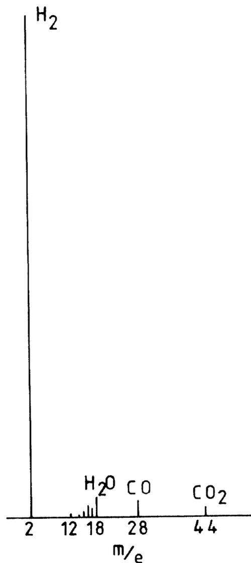
Fig. 5 : The residual gas spectrum in a powered cavity assembly.
