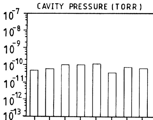
Fig. 2: A pressure profile from a set of 8 unpowered cavity assemblies.
