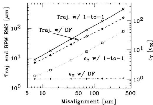
Figure 6: 1-to-1 and DF correction vs. the misalignments.
