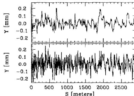
Figure 1: Trajectory after correction in the NLC.
