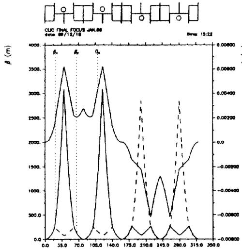
Figure 2: Lattice and orbit functions of the CCS
