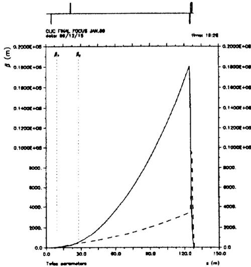
Figure 1: Lattice and orbit functions of the final telescope
