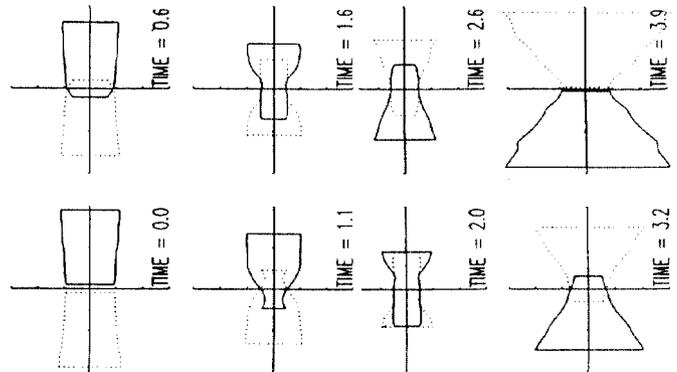
Figure 5: Beam-Beam effect for head-on collision of two bunches at the IP of CLIC
