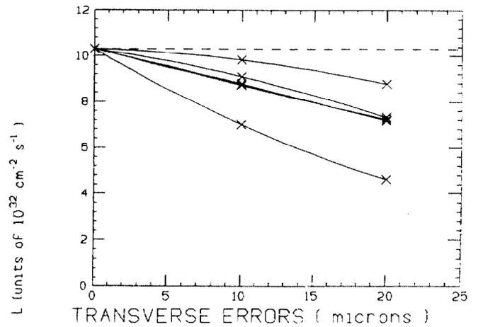
Figure 6: Reduction of luminosity with RMS misalignment error of magnetic elements and pick-ups in the CLIC FFS
