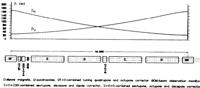
Figure 1: Layout of the LHC Standard Half-Cell
