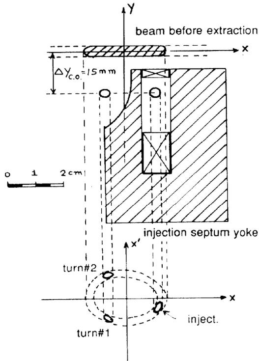
Fig. 4 Geometry of magnetic injection septum. Top part shows situation in *real* space; bottom part shows  $(x, x')$  phase space at injection location.
