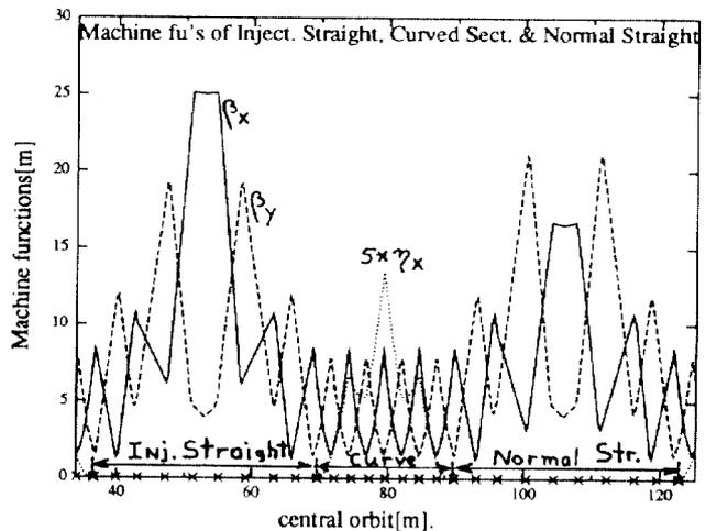
Fig. 3 Machine functions of East (Injection area) and South part of AmPS
