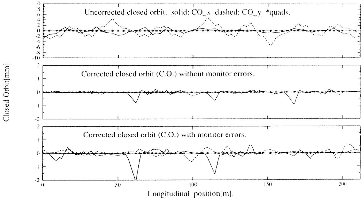
Fig. 5 Orbit correction and misalignment errors (numbers in text): Top: UNcorrected closed orbit (C.O.) Middle: Corrected C.O. without misaligned monitors and reading errors. Bottom: Corrected C.O. including misaligned monitors and reading errors
