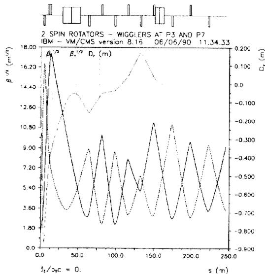
Figure 2: Orbit Functions in the Spin Rotator
