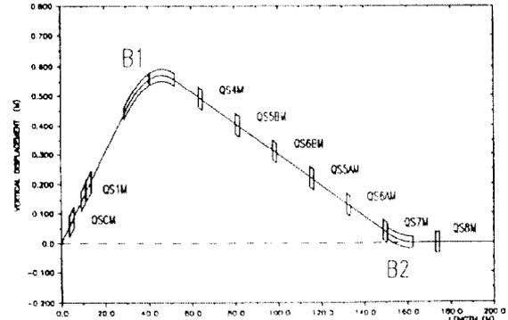
Figure 1: Layout of the Richter-Schwitters Spin Rotator
