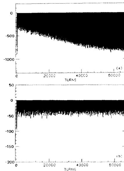
Figure 7: The plots of a simulation result for the synchrotron radiation signal. The top plot is the result for coherent damping. The bottom one is the result for decoherence. To produce the decoherent effect, we add an octupole magnet to the lattice which was used to produce the top result.
