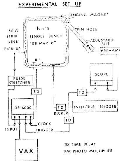
Figure 3: A schematic drawing of the experimental set up for the head-tail damping rate measurement.
