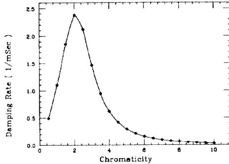
Figure 2: The chromaticity dependence of the damping rate obtained by performing the summation in Equation 1 for the parameters of Aladdin. In this plot the bunch current is 2.3 mA and the bunch length is 1.5 meters.
