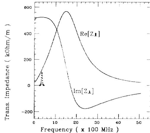
Figure 1: The broad band transverse impedance of Aladdin. The '+' curve is the spectrum of  $h_0$  which is a gaussian distribution and the central frequency is the chromaticity frequency  $\omega_\xi$ . In this figure,  $\omega_\xi = 0.356$  GHz,  $\xi = 0.5$ .
