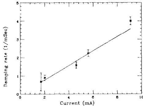
Figure 5: The measurement of the current dependence of the damping rate. The line is predicted by the theory.
