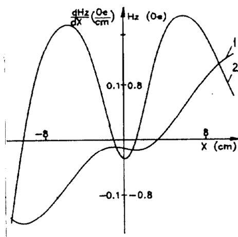
Fig. 1. Magnetic field (1) and gradient (2) distributions introduced by the octupole winding.
