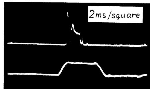
Fig. 3. Oscillogram of a gradient winding current pulse (bottom trace), time structure of the external beam, 2 ms/square.
