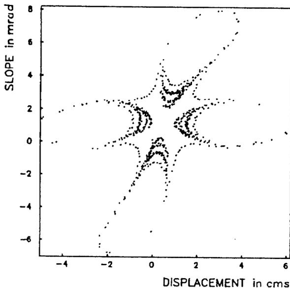
Fig. 2. Computed phase plot of the electron resonance betatron oscillation.
