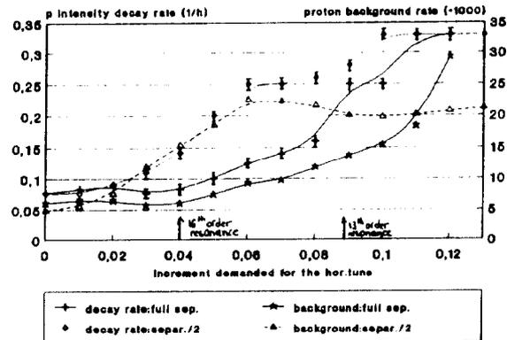
Fig.4: proton intensity decay rate and proton background rate as a function of the horizontal tune.
