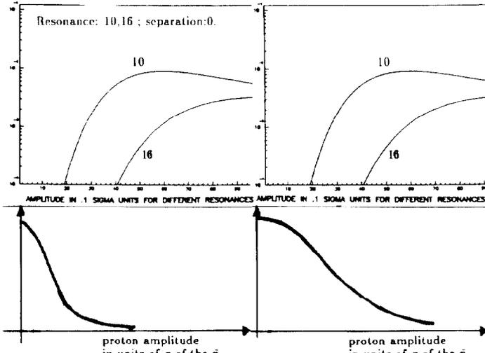
Fig.3: transverse distribution of the protons and resonance width functions seen by the proton beam before and after the scraping. The horizontal abscissa of both transverse distribution of the protons and resonance width is the proton amplitude in units of the r.m.s.  $\bar{p}$  beam size.
