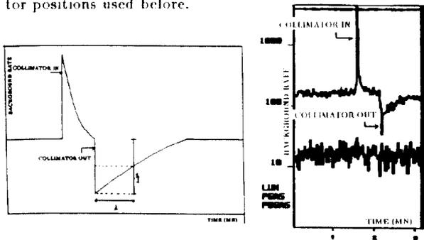
Fig.5: schematic drawing of the proton background rate as a function of time and the observed proton background rate as a function of time.
