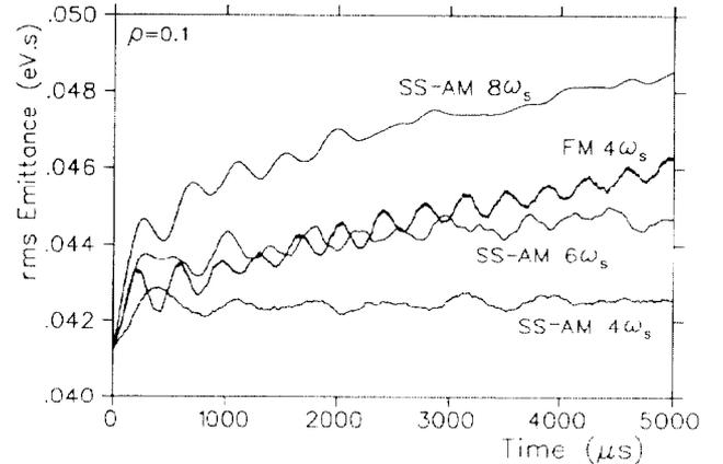
Fig.3 : Comparison of SS-AM with in-phase FM.
