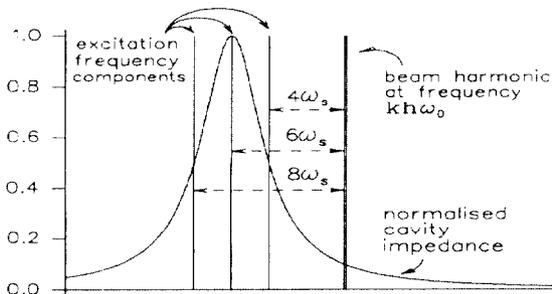
Fig. 5 : Power spectra for triple-frequency SS-AM.
