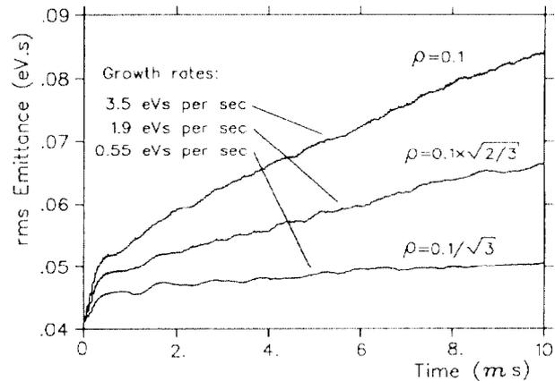
Fig. 6 : Triple-frequency excitation for various signal power.
