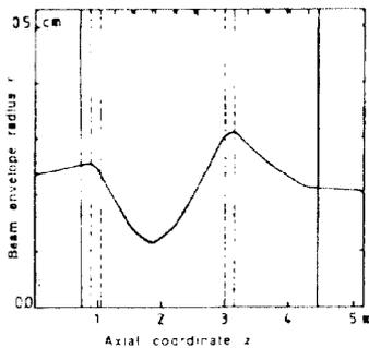
Fig.2 Beam envelope (including 95% of the beam) through a cryostat housing 8 resonators and 2 solenoids (dotted lines)
