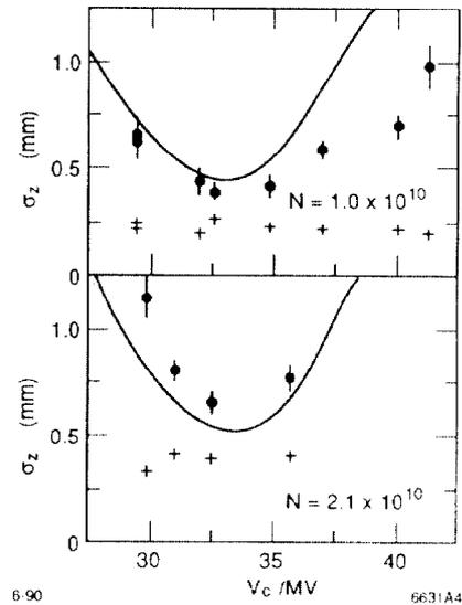
Fig. 4. The bunch length  $\sigma_z$  measured as function of compressor voltage  $V_c$  for bunch populations  $N = 1.0 \times 10^{10}$  (top) and  $2.1 \times 10^{10}$  (bottom). (The data is given by the circles.) Also shown is the results with Sector 9 turned off (+). The calculated bunch length is given by the curve.
