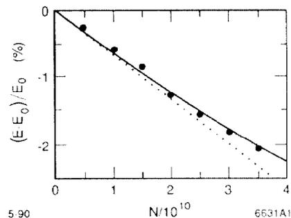
Fig. 1. The change in final beam energy measured as function of beam current (the circles). The compressor voltage  $V_c = 29$  MV, the reference energy  $E_0 = 47$  GeV. The solid curve gives the calculation results, the dotted line the calculated results assuming there is no bunch lengthening in the damping rings.
