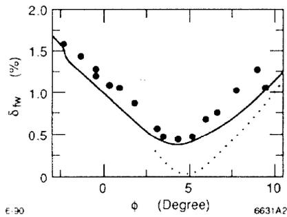
Fig. 2. The spectrum width  $\delta_{fw}$  measured at the end of the SLC linac as function of overall linac phase for  $N = 1.5 \times 10^{10}$  (the circles). Also shown on the plot are the calculated results when the resolution of the hardware (0.15%) is included (the solid curve) and when it is not (the dots). Here  $V_c$  is assumed to be 27.4 MV.
