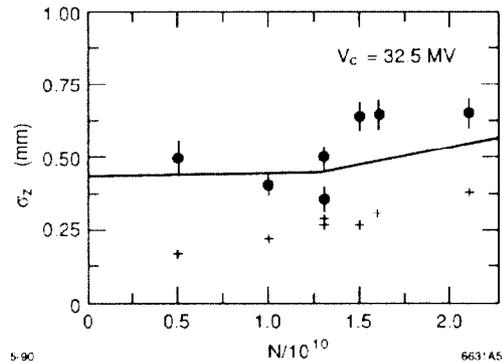
Fig. 5. The bunch length  $\sigma_z$  measured as function of current (the circles). The compressor voltage  $V_c = 32.5$  MV. Also shown are the measurements with Sector 9 off (+) and the calculated bunch length (the curve).
