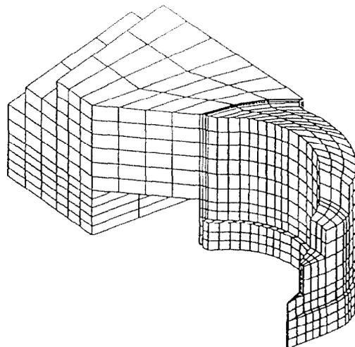
Fig. 3 Finite element model of the EULIMA magnet
