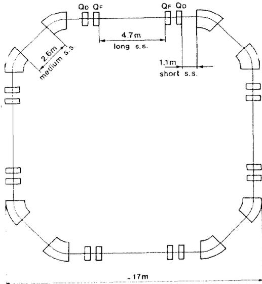
Fig. 2 An arrangement of EULIMA synchrotron lattice
