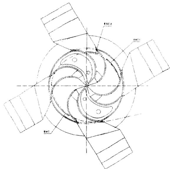
Fig. 1 Lay-out of the separated sector superconducting cyclotron
