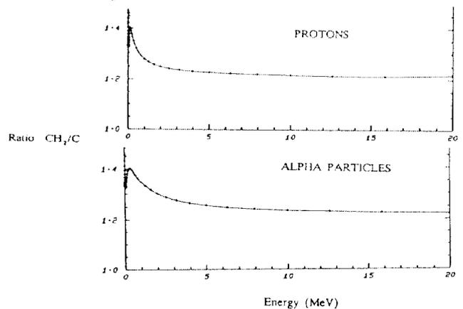
Fig. 5. Energy dependent stopping power ratios for protons and alpha particles in CH<sub>2</sub> and C.
