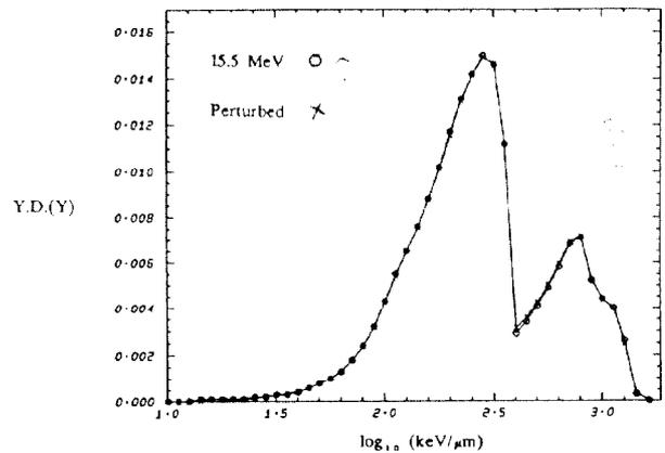
Fig. 4. Calculated microdosimetric responses of a carbon detector exposed to 15.5 MeV neutrons with and without perturbation.
