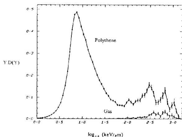
Fig. 6. Monte Carlo calculation of the microdosimetric response of a  $\text{CH}_4$  filled ( $2\mu\text{m}$ ) polythene counter exposed to 15.5 MeV neutrons
