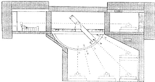
Fig. 3. 90° Rotating Magnet System for Beam Delivery to Three Treatment Rooms
