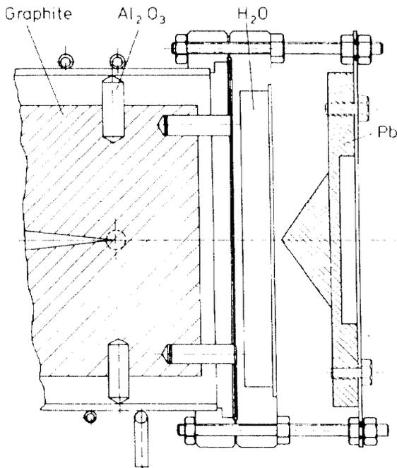
Fig.1. Schematic view of beam stop with Pb-flattening filter
