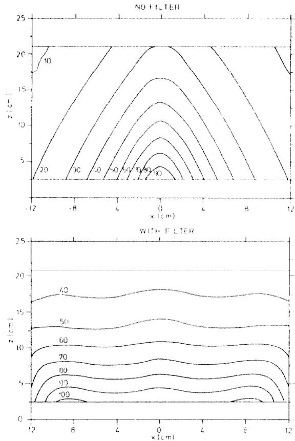
Fig.2. Isodose charts measured in the irradiation phantom (x : distance from center z : depth in phantom)
