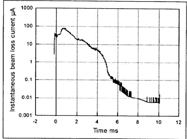
Fig. 3. Instantaneous beam loss current with time.
