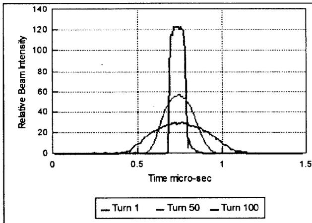
Fig. 6. Chopped beam pulse debunching over 100 turns.
