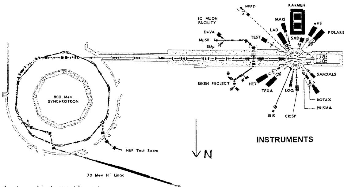
Fig. 1 ISIS accelerator and instrument lay-out.
