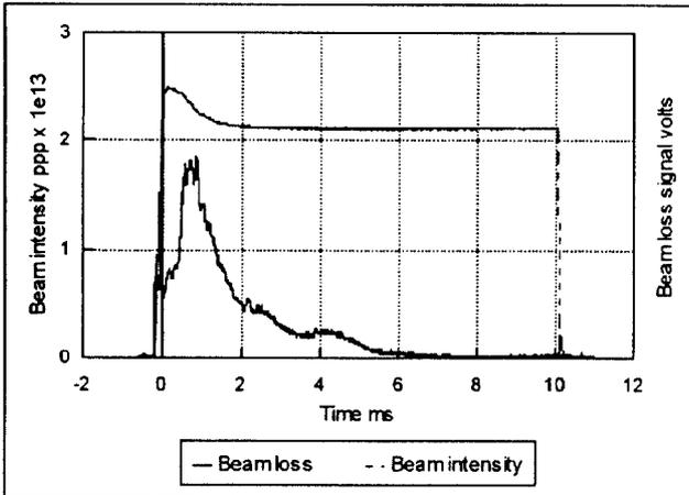
Fig. 2. Beam intensity and beam loss monitors sum signal during acceleration.
