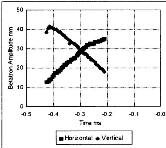
Fig. 5. Horizontal and Vertical betatron amplitudes during injection.
