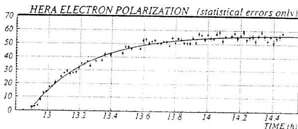
Figure 6: Longitudinal polarisation in the HERA electron ring. The vertical direction of the electron spin is turned into the longitudinal one during the passage of the experimental area.
