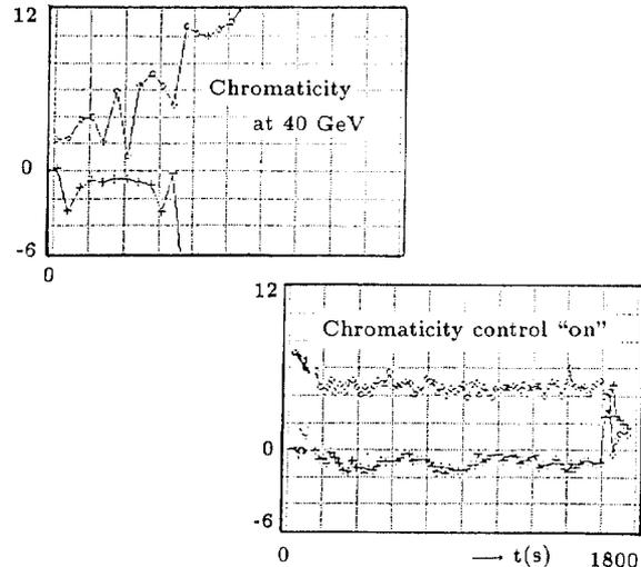
Figure 5: Time dependent behavior of the persistent current contribution to the chromaticity in the HERA proton storage ring. In the second part of the plot the effect of the persistent current decay is counteracted by an automated control of the chromaticity.
