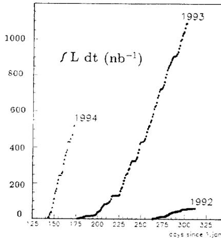
Figure 2: Integated luminosity of Hera measure by the experiment Zeus during the run periods 1992,1993 and 1994
