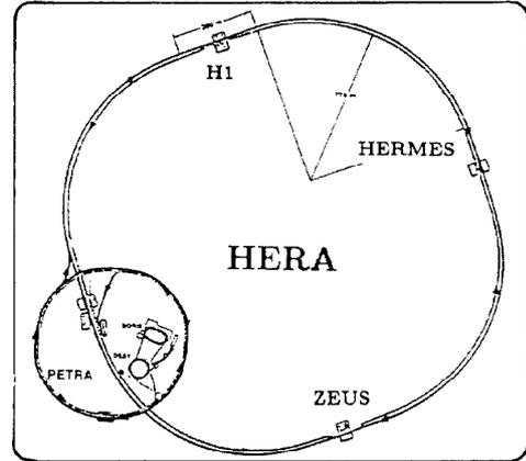
Figure 1: Geometry of the electron proton collider HERA. The bunches of the proton and electron machine collide at the interaction points “North” and “South” where the detectors of the experiments ZEUS and H1 are located. The straight section “East” is prepared for the third experiment Hermes which will be installed in winter 1994/95.
