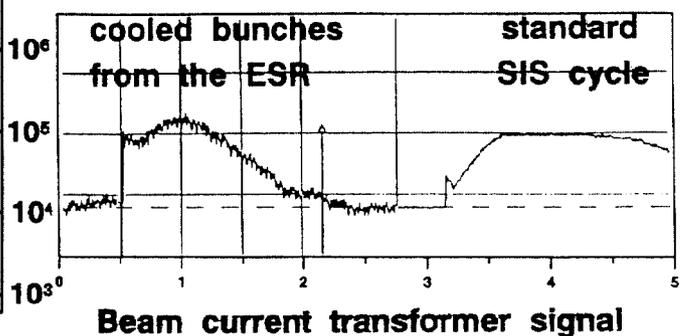
Figure 4: Transfer of a 200 MeV/u cooled ESR beam to the SIS. On the left side the beam transformer signal shows acceleration of the cooled ESR beam to 500 MeV/u and slow resonance extraction, on the right a standard SIS cycle follows with acceleration of a 11.4 MeV/u Unilac beam to 400 MeV/u.
