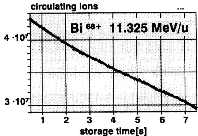
Figure 2: Beam life time for  $Bi^{68+}$  ions at 11.4 MeV/u injection energy and  $4 \cdot 10^{-11}$  mbar average SIS pressure.
