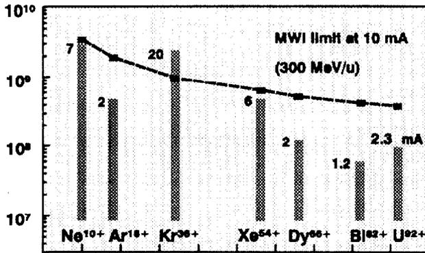
Figure 7: ESR coasting beam intensities by the end of 1993. The present intensity limit caused by transverse microwave instabilities at 10 mA is indicated
