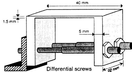
FIGURE 4 : Schematic drawing of the new "U-shaped" silicon crystal, cut out of a block of silicon, including the "feet" needed to bend it. Bending is achieved with two differential screws.
