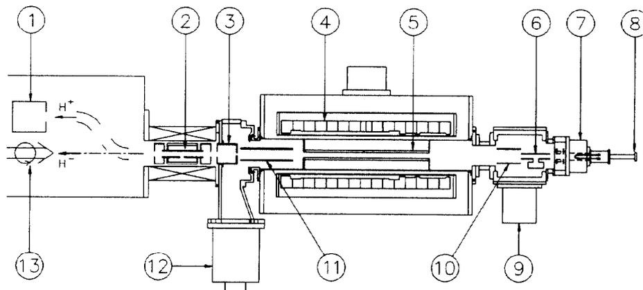
Fig. 1. Setup for spin-exchange polarization measurements. 1) Lyman-alpha polarimeter, 2) ionizer Rb cell, 3) Sona transition region, 4) 10 kG S.C. solenoid magnet, 5) 60 cm optically-pumped Rb cell, 6) neutralizer Rb cell, 7) duoplasmatron, 8) window for probe laser, 9) turbopump, 10–11) deflection plates, 12) cryopump, 13) pump laser light.
