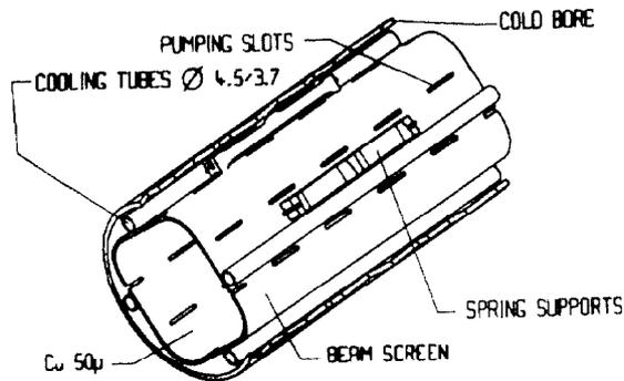
Figure 1. LHC dipole beam screen
