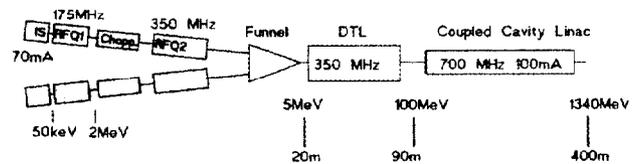
Fig. 14 Scheme of a high current ESS-injector linac
