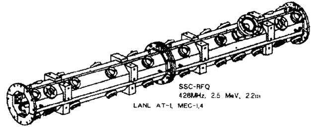
Fig. 7 The SSC-RFQ cavity
