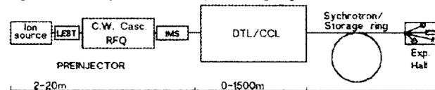
Fig. 1 Scheme of a high intensity accelerator system
