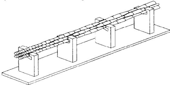
Fig. 11 Scheme of the DESY 4-Rod RFQ structure
