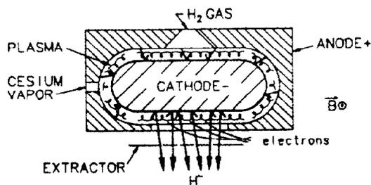
Fig. 2 Basic magnetron source configuration
