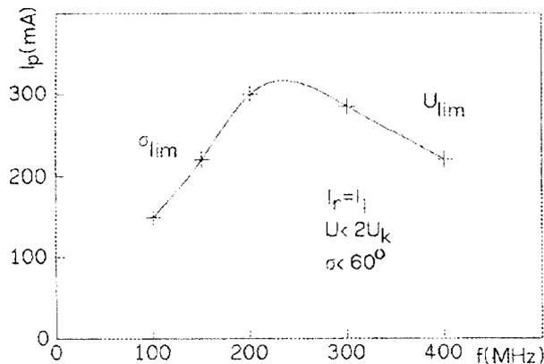
Fig. 7 Proton Current as function of the operating frequency
