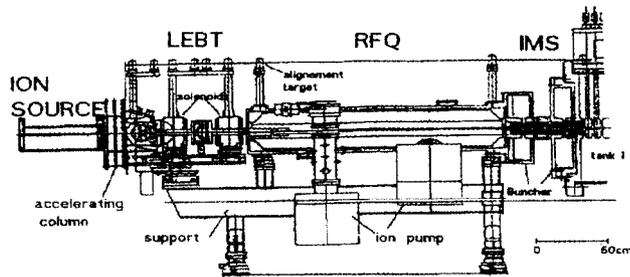
Fig. 12 Layout of the CERN RFQII injector
