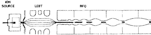
Fig. 6 Scheme of a RFQ injector
