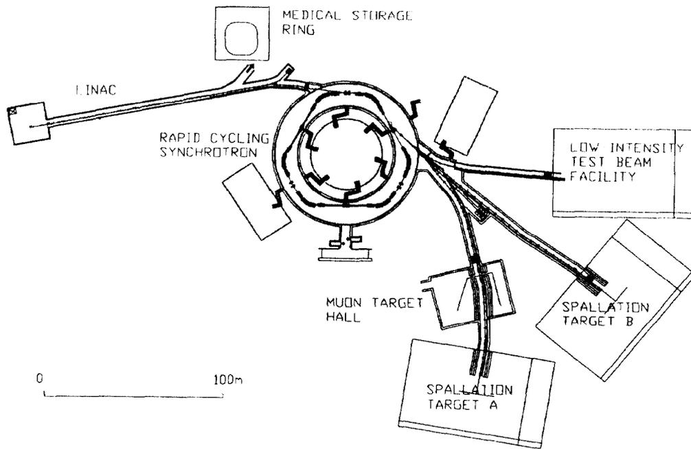
Fig. 1: Layout of AUSTRON
