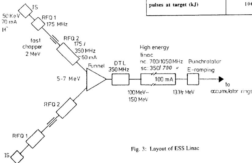
Fig. 3: Layout of ESS Linac
