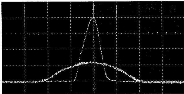
Figure 3. Bunch shape before (long ), during (short ) and after (long and superposed) bunch compression (time scale: 50 ns/div).
