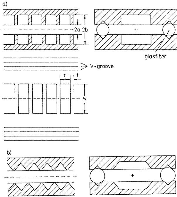
Figure 2. The double-sided muffin-tin structure.
