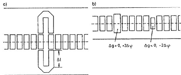
Figure 4. Muffin-tin with a) delay lines, b) periodically changing cavity length.
