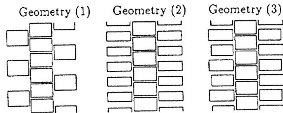
Figure 3. Side-coupled muffin-tin structures with (1) alternating, (2) symmetrically arranged off-axis cells and (3) with broken symmetry.
