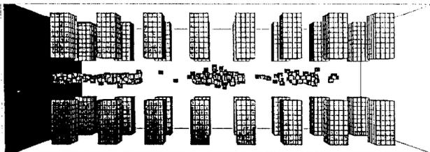
Figure 6. MAFIA simulation of acceleration and bunching of a low  $\beta$  beam.
