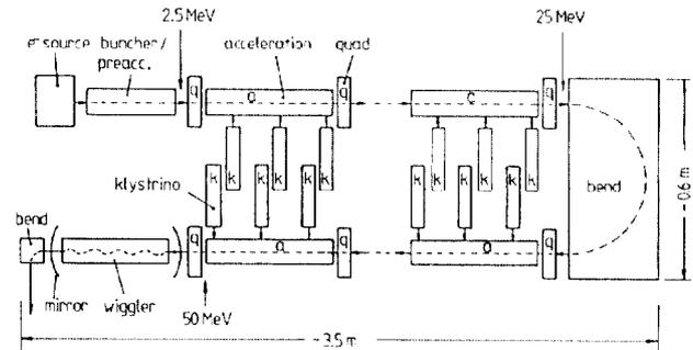
Fig. 1 Conceptual design of an integrated mm-wave radiation source (IMIRAS)
