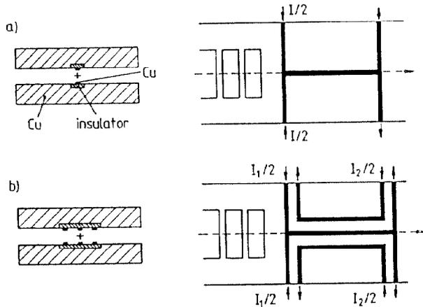
Figure 8. Integrated pulsed wire magnets for focussing in a) the vertical plane and b) in both planes.
