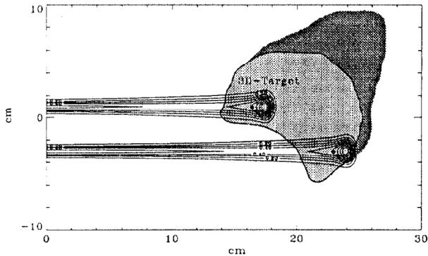
Figure 3a. Principle of the spot scanning technique: through the weighted superposition of individual spots . . .
